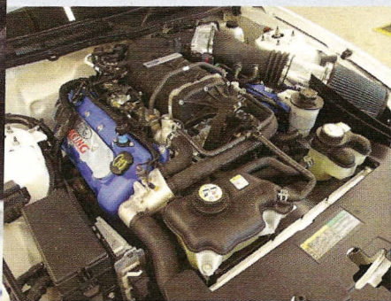
Four-valve motors love superchargers. All that valve area is just waiting for 8 or 10 psi of pressure to stuff loads of air and fuel into even smallish 5.4L (330ci) cylinders. The iron-block package mounts stock heads, a TVS supercharger, and an SFI damper, along with a twin-bore 62.5mm billet throttle body, long-tube headers, and an A/C-delete pulley. That's it.
