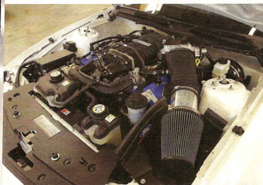
The cold-air package picks up air toward the front of the fascia rather than from the hoodcoop.
