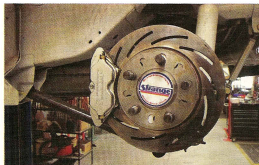
Strange supplied the gears, 35-spline axles, and rear disc brakes for the 9-inch.
